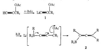
Formation of the desired lithium salt (1) was accomplished without interference by the acetate group by reaction of the ethynylalkanol acetate with n-butyllithium at low temperature (-78 or -120 °C). Addition of a trialkylborane followed by warming to room temperature and then protonation with acetic acid results in the formation of an allene.<sup>2,5,6</sup> The overall
